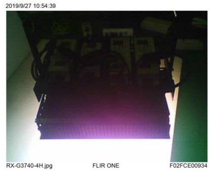
RX-G3740-4H 450W Surface temperature test
